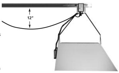
Drive Motor can travel its full distance without restriction. We recommend that there be at least 12 inches distance from the bottom of the rail to the center of the power cords arc when the cord's are fully extended and fasten both cords to the bottom of the Drive Motor. You can fasten to either of the two holes or the eye screw described earlier. Please do not fasten to the Motors Wires.
