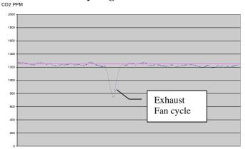
The PPM-2a's *Artificial Intelligence* (Fuzzy Logic) behaves as though you have a trained operator in your growing area to monitor the  $CO_2$  level and release more  $CO_2$  only when required. PPM-2a users can expect to have their  $CO_2$  level kept within 25PPM of their desired set point. The PPM-2a automatically "learns" how to best maintain the set point as it operates. This will result in a huge savings when using compressed  $CO_2$  gas compared to standard on / off controllers.
